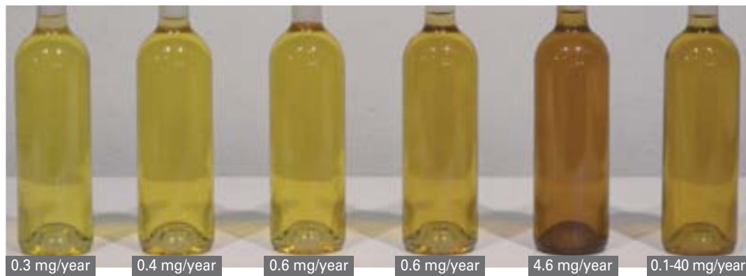
■ Figure 2: Illustration of the impact of stoppers' OTR on the intensity of yellow-orange tint of a Sauvignon Blanc wine (M-ap) after 10 years of bottle aging (ranking of samples as a function of OTR values in Table 1 ).
